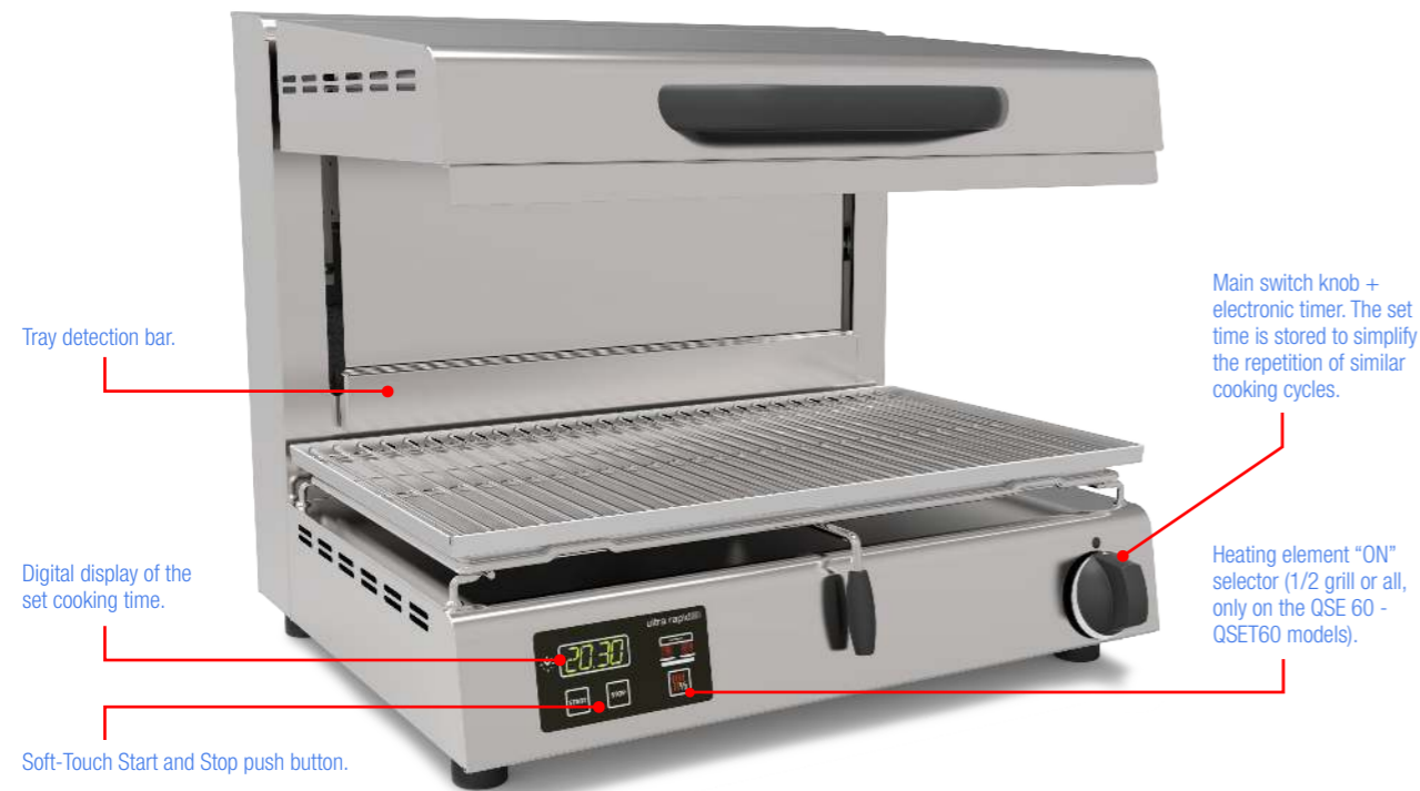
QSET60 - QSE60: GN1/1 cooking plate with the possibility to heat up only half of the surface.
